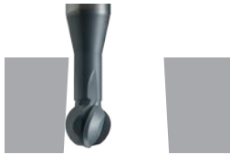
⑤ Undercut (Taper Hole)
