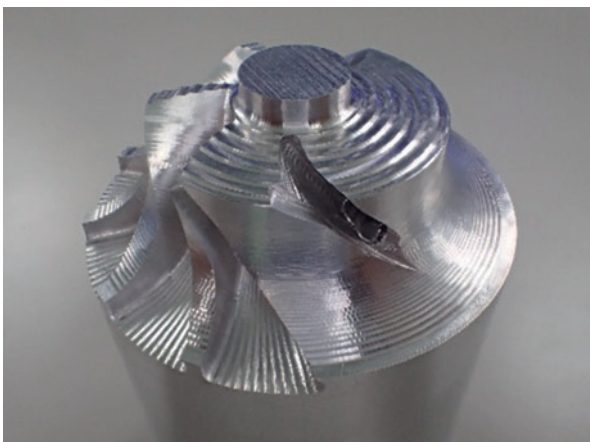
Breakage During Grooving
